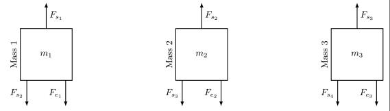
We now introduce the vector  $\mathbf{y}(t)$  to store the net force on each mass. When writing the individual entries of  $\mathbf{y}(t)$  we will assume that positive forces result in positive displacements. Since we've oriented positive displacement in the downward direction, we also orient positive force in the downward direction.
