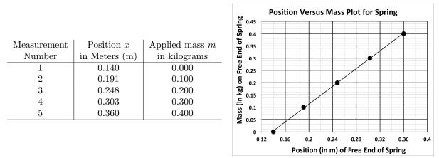
From this data, we can calculate  $u_i$ , the displacement of movable end of spring in measurement i. We can also create a mathematical model in the form
