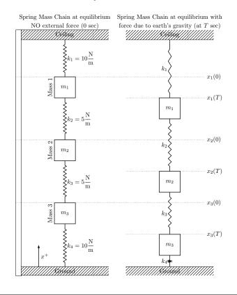
16. Recall that the initial position vector  $\mathbf{x}_0$  and the mass vector  $\mathbf{m}$  store the positions, measured in meters, of each mass at equilibrium when t = 0 and the mass measurements, measured in kg, respectively. Suppose we measure
