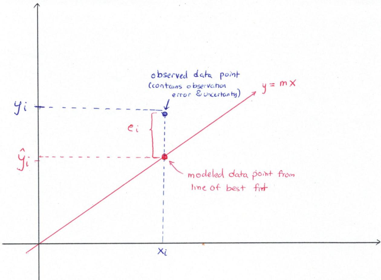
We defined the error between our collected data output  $y_i$  and our modeled output  $\hat{y}_i = mx_i + b$  to be
