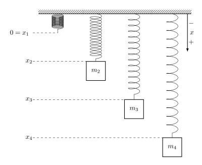
In order to model the relationship between the displacement of the movable end of the spring and the internal force stored in the spring, we introduce two  $4 \times 1$  vectors given by
